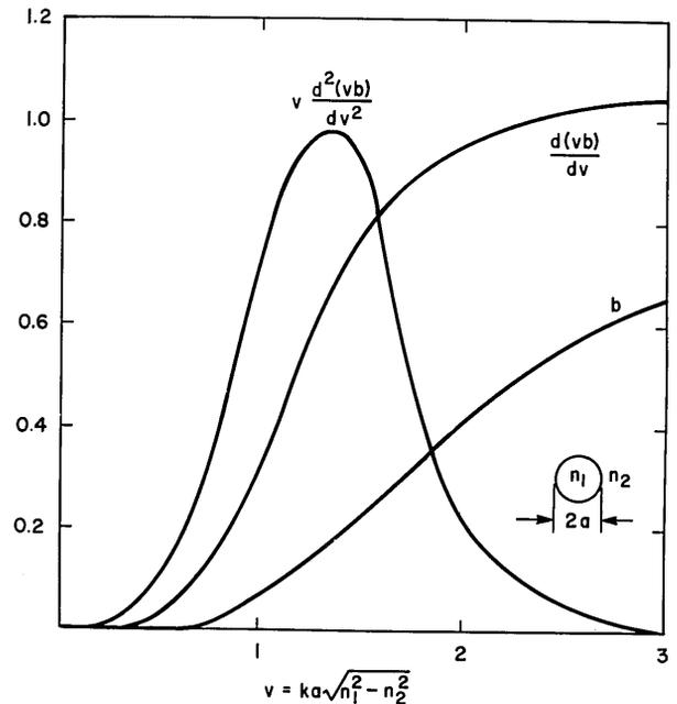
Fig. 2. Waveguide parameter  $b$  and its derivatives  $d(vb)/dv$  and  $vd^2(vb)/dv^2$  as a function of the normalized frequency  $v$ .
