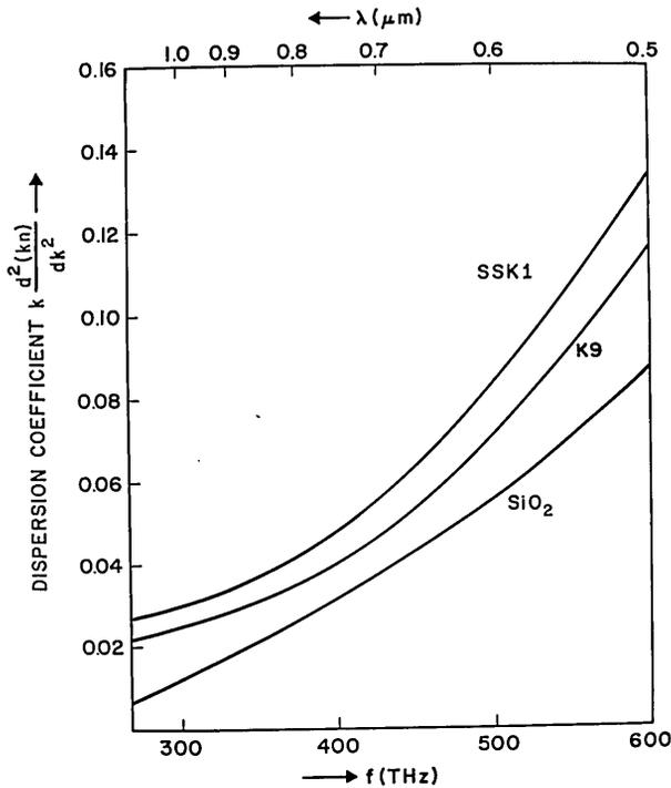
Fig. 3. Dispersion coefficient  $kd^2(kn)/dk^2$  as a function of frequency for fused silica ( $\text{SiO}_2$ ) and the Schott glasses K9 and SSK1.
