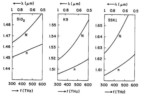
Fig. 1. Refractive index  $n$  and group index  $N = d(kn)/dk$  as a function of frequency for fused silica ( $\text{SiO}_2$ ) and the Schott glasses K9 and SSK1.
